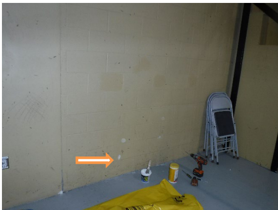
Sample 17: drilled hole west wall by bleachers in cinderblock wall (empty)
