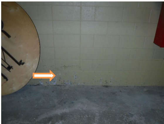
Sample B: Yellow paint over red paint; north wall middle of wall (1200 ppm)
